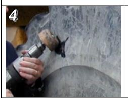
Grind the damaged area using a rubber grinding disk like the Rubber Exterminator. It is imperative you get a rough texture to allow for good adhesion.
