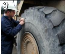
Skive out the rubber around the rip or tear. Be careful not to damage the steel radial of the tire with the blade
