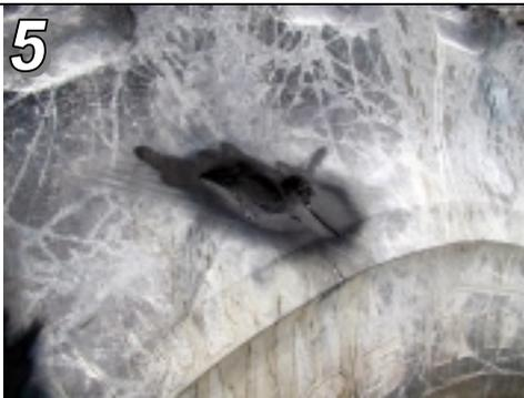
5 Paint the damaged area with Eli-Bond FR704 adhesion promoter. Allow to dry until it is very "finger tacky". Don't apply FR909 to soon. You will trap solvents which will reduce the bonding strength
