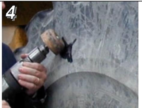
4 Grind the damaged area using a rubber grinding disk like the Rubber Exterminator. It is imperative you get a rough texture to allow for good adhesion.
