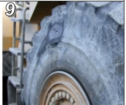
9 Allow 8 hours for Eli-Flex to cure. Buff as needed. See Tech Specifications for curing time at varying temperatures
