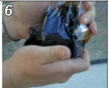
6 Open Eli-Flex FR909 kit, remove the spine and mix the two components together for 2-3 minutes or until warm. See "Six Easy Steps to Belt Repair" for more detailed instructions.
