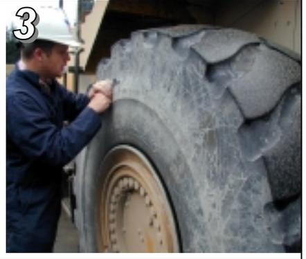
3 Skive out the rubber around the rip or tear. Be careful not to damage the steel radial of the tire with the blade
