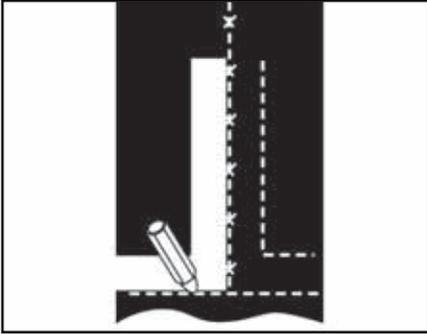
**1.** Square belt ends using centerline method.
